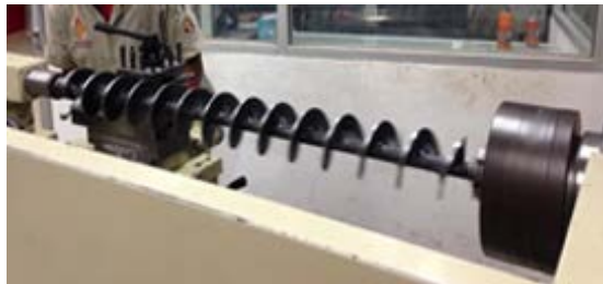
Fig. 2. The 5-inch screw blade is connected to the 1 inch shaft.
