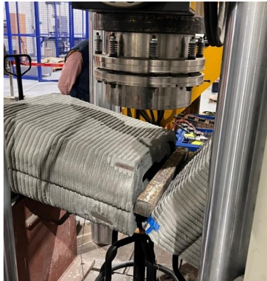
Fig. 9. 3DCP bridge segment after failure.
