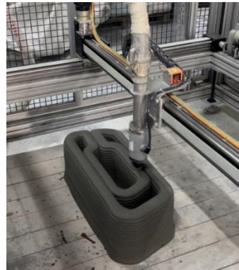
Fig. 5. The bridge segment during printing.
