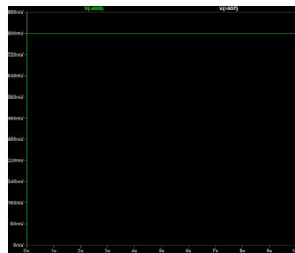
Fig. 8. Input (0.8V-green) and output (0V-white) waveforms.
