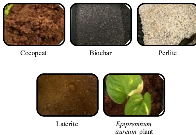
Fig. 1. Four filter media used for filtration of rainwater.
