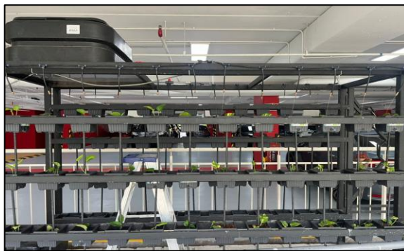
Fig. 2. The green wall setup used for rainwater filtration.
