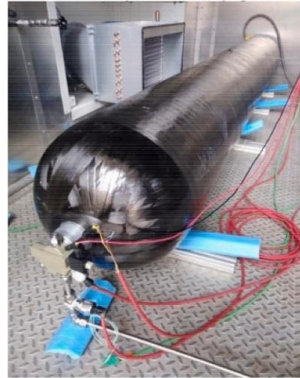
Fig. 1. Comet type III hydrogen storage cylinder [18].
