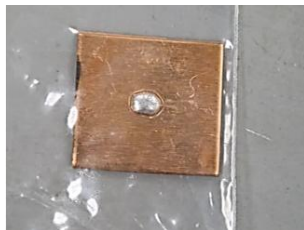
(c) SnBi/Cu soldered piece.
