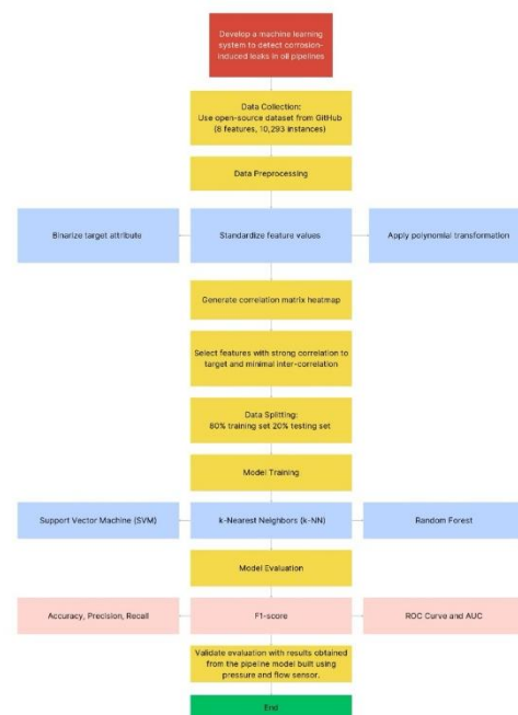
Fig. 1. Main flow chart of the methodology for developing a machine learning system for detecting oil pipeline leakage.
