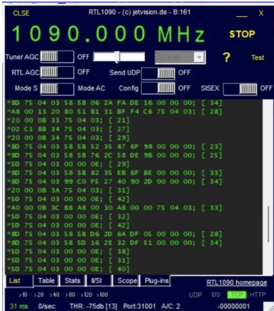
Fig. 10. RTL-1090 software detecting ADS-B signals.
