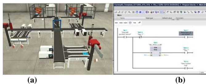
Fig. 6. (a) Overview of the 3D rendering and simulation; (b) Run block diagram coded for the simulation.
