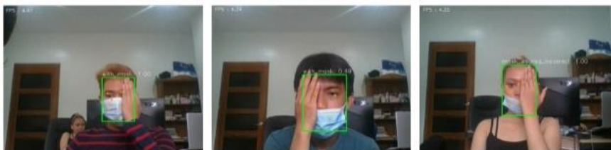
Fig. 6. Occlusion with classification (a) partial occlusion with face mask (b) half face occlusion with incorrect wearing (c) half face occlusion with incorrect wearing.
