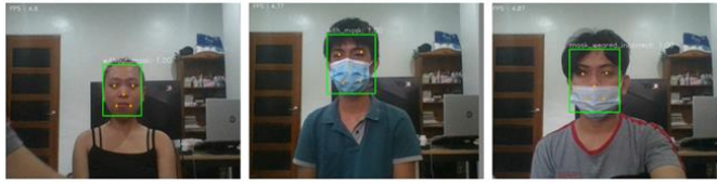
Fig. 5. Face mask classification (a) no face mask, (b) correct wearing of face mask, and (c) incorrect wearing of face mask.
