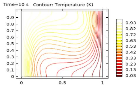
Fig. 3. Thermal contours for  $Ra = 2 \times 10^4$  and  $Rs = 0$ .
