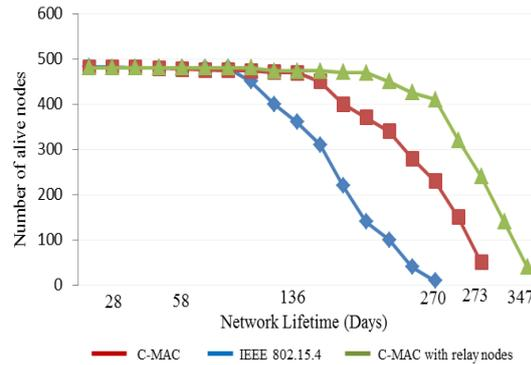
**Fig. 24. The effect of different protocols on the percentage of alive nodes of 482 nodes.**
