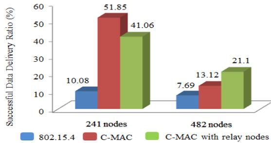
Fig. 22. The comparison of successful data delivery ratios of 241 and 482 nodes.
