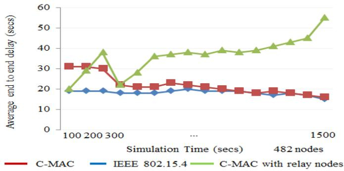
Fig. 19. The effect of C-MAC on average end to end delays of 482 nodes.
