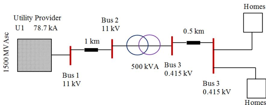
**Fig. 1. The design of the power distribution grid of 1500 MVA using ETAP simulator.**
