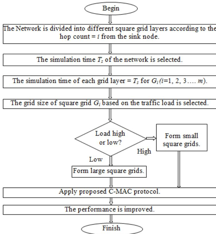
**Fig. 4. The flowchart of the proposed C-MAC protocol for WSN.**
