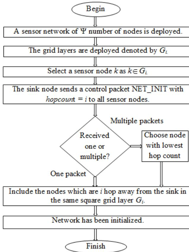
Fig. 3. The flowchart of the network initialization phase.
