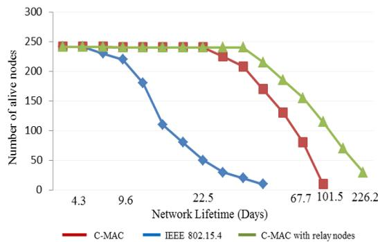
Fig. 23. The effect of different protocols on the percentage of alive nodes of 241 nodes.
