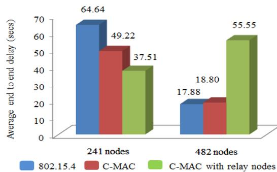
**Fig. 17.** The comparison of average end to end delays of 241 and 482 nodes.
