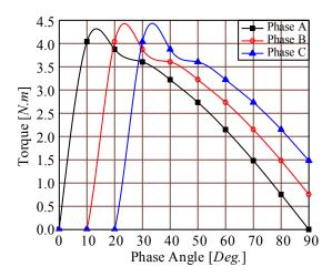
Fig. 7. Three phase static torque.
