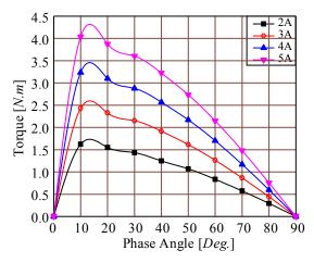
Fig. 6. Current torque characteristics.
