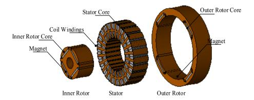
Fig. 1. Double rotor interior permanent magnet motor (exploded view).
