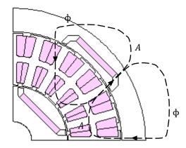
Fig. 2. Operating principles of DRFAPM motor.
