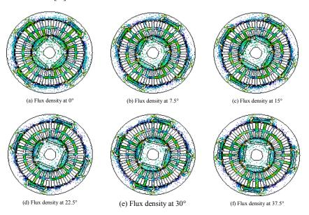
Fig. 4. Flux flow for various rotational angle.
