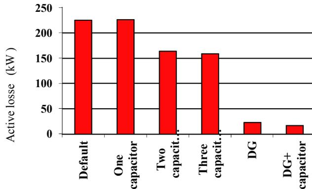
Fig. 8. Active Power Losses Comparison in Different Cases.
