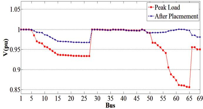
Fig. 7. Voltage Profile of 69-Bus System (Scenario II) before and after Placement.
