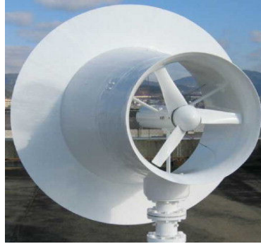
Fig. 1. Prototype Wind Turbine with a Flanged Diffuser Shroud (500 W). The Rotor Diameter, D , is 0.72 m. The Area Ratio \mu (Outlet area/Inlet Area) of the Diffuser is 2.35. [9]
