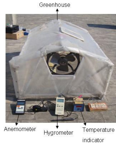
Fig. 1. Experimental Set-up of Greenhouse Papad Drying under Forced Convection Mode.
