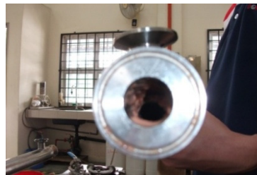
(b) Lab-scale Concentric Tube-Pasteurizer.
