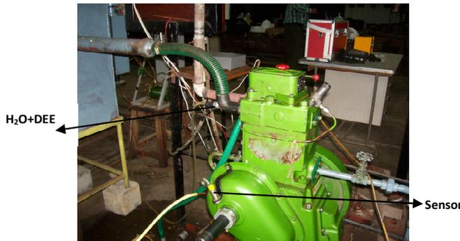
**Fig. 1. Diesel Engine Test Rig with Water-DEE Injection Equipment.**
