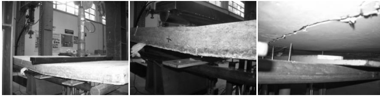
Fig. 11. Crack Occurred at the Bottom of Slab when Subjected to Bending Test.
