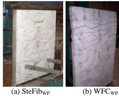
Fig. 9. Failure Visualisation of SteFib WP and WFC WP .
