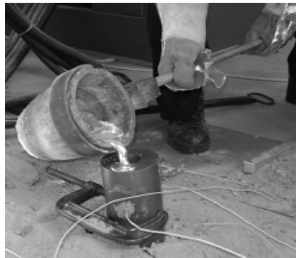
Fig. 4. Pouring MMCs Melt into the Permanent Mould.
