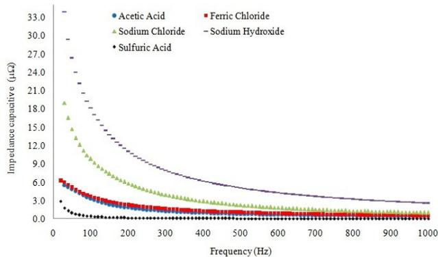
**Fig. 9. The Impedance Capacitive of a Mortar-Filled Sensor Immersed in Different Solutions.**
