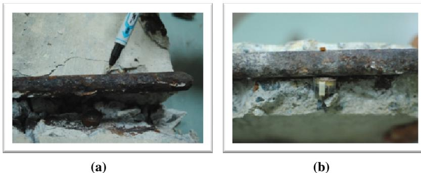
**Fig. 12. Visual Inspection of Corroded Rebar: (a) Specimen Exposed to Indoor Environment. (b) Specimen Exposed to Corrosion Chamber.**
