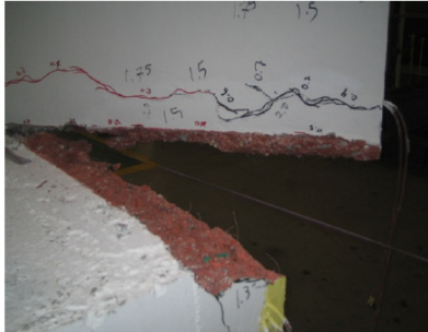
e) Cracks Appear at the Upper Part of the Wall.
