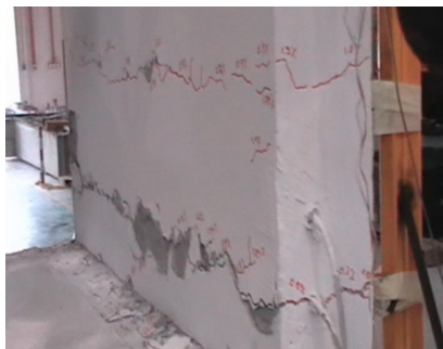
f) Spalling of Concrete at the Anchorage Location and Hairline Cracks at the Top of the Wall.
