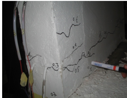
d) Cracks intensified at the Front Face of the Wall at the Anchorage Location.
