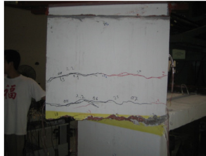
f) Concrete Spalling Starts to Appear at the Back of the Connection.
