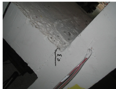
b) Minor Hairline Cracks Appearing at the Side at the Connection at 0.3% Drift.
