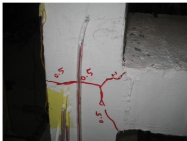
c) Diagonal Cracks Propagate across the Connection.
