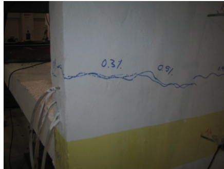
b) Minor Hairline Cracks Appearing at the Back at the Wall at 0.3% Drift.
