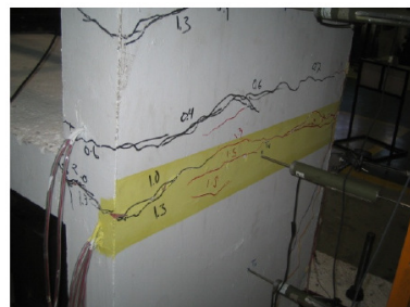
d) Cracks Intensified at the Back of the Connection.
