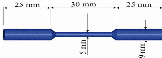
**Fig. 2. Cylindrical Tensile Test Piece.**
