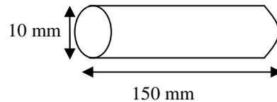
**Fig. 1. Cylindrical Wooden Pattern.**
