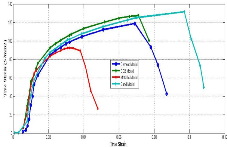
**Fig. 3. True Stress against True Strain.**
