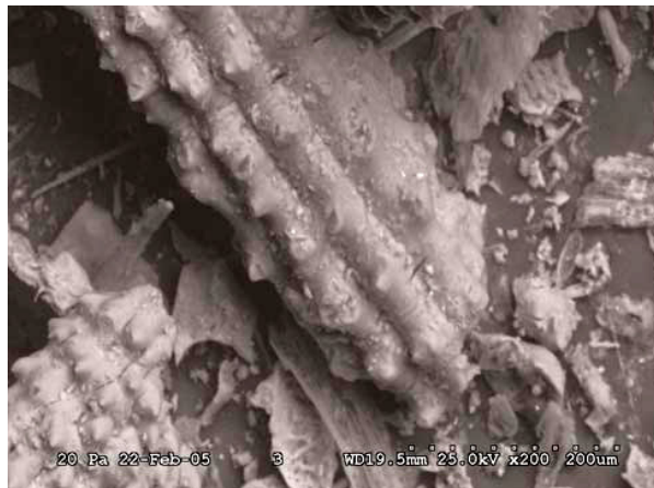
Fig. 4. Typical SEM Image of RHA Particle showing Honeycombed Structure.
