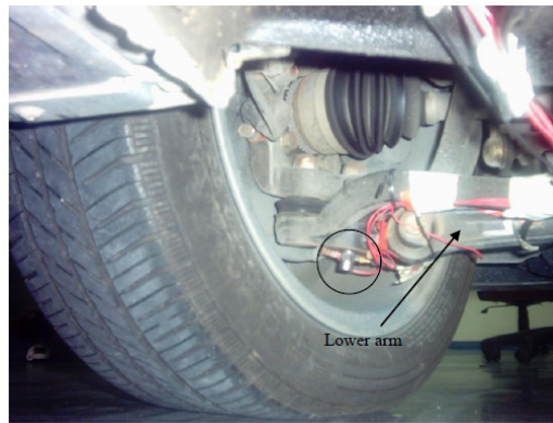
Fig. 5. Accelerometer Mounted at the Lower Arm (before Damper).
