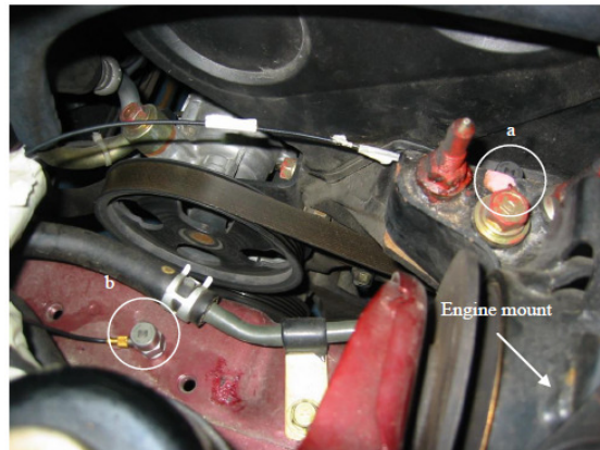
Fig. 2. Accelerometer Positions: a) Before the Engine Mount, b) After the Engine Mount.
