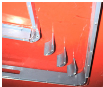
Fig. 1. Blade Row attached to One Side of End Wall.
