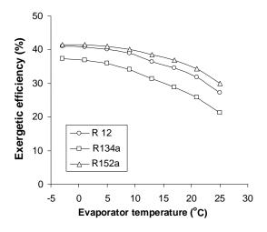
Fig. 4. Variation of Exergetic Efficiency with Evaporator Temperature.
