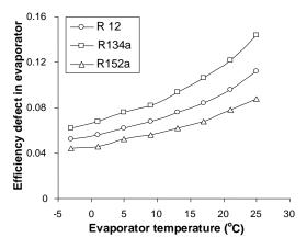
Fig. 8. Variation of Efficiency Defect in Evaporator with Evaporator Temperature.
