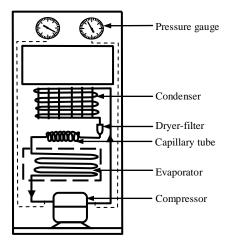
Fig. 2. Schematic Diagram of Experimental Refrigerator.
