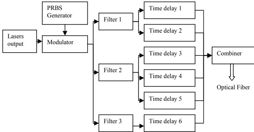
Fig. 2. Encoder Design of Optical CDMA System.
