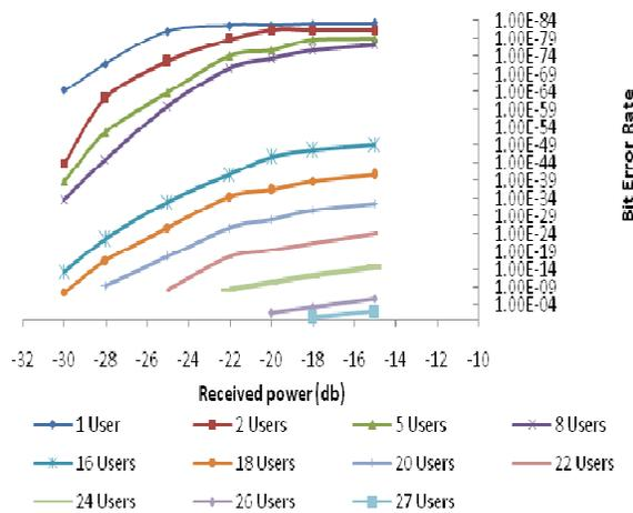
**Fig. 16. Bit Error Rate versus Received Power for Different Number of Simultaneous Users for 1 Gbps SCOOC Based OCDMA System.**
