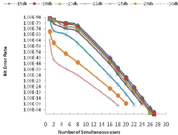
**Fig. 15. Bit Error Rate versus Number of Simultaneous Users at Different Received Power for 1 Gbps SCOOC Based OCDMA System.**
