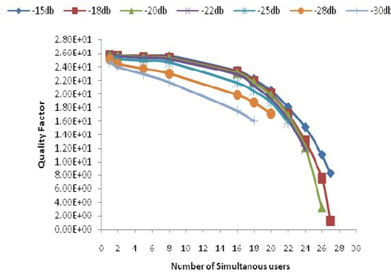
**Fig. 17. Quality Factor versus Number of Simultaneous Users at Different Received Power for 1Gbps SCOOC Based OCDMA System.**
