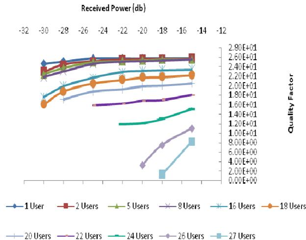
**Fig. 18. Quality Factor versus Received Power for Different Number of Simultaneous Users for 1Gbps SCOOC Based OCDMA System.**
