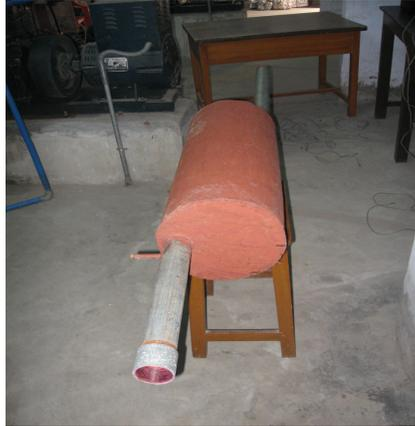
**Fig. 4. Developed Reactive Muffler.**
