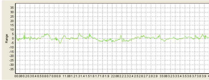
**Fig. 1. Surface Roughness Profile Chart, Cutting Speed ( $V=112$  m/min), Feed Rate ( $f=0.2$  mm), Depth of Cut ( $doc=1.5$  mm), Surface Roughness ( $R_a=1.509$   $\mu\text{m}$ ).**
