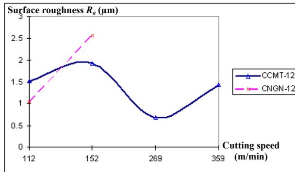
**Fig. 2. Cutting Speed vs. Surface Finish for Turning Nickel Based Alloys Haynes -276 Using CCMT-12 and CNGN-12 Inserts at a Feed Rate 0.2 mm/rev and Depth of Cut 1.5 mm.**
