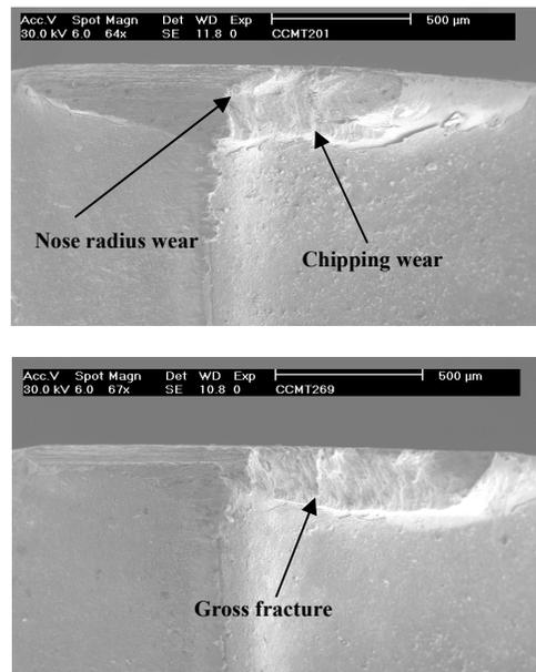
**Fig. 4. SEM Images Showing the Wear of the CCMT-12 after Machining Nickel Based Alloys, Haynes-276 at (a) 201 m/min, (b) 269 m/min.**
