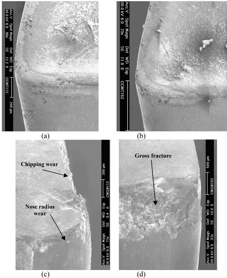
**Fig. 3. SEM Images Showing the Wear of the CCMT-12 after Machining Nickel Based Alloys, Haynes-276 at (a) 112 m/min, (b) 152 m/min, and CNGN -12 after Machining Nickel Based alloys, Haynes-276 (c) 112 m/min and (d) 152 m/min Cutting Speeds.**
