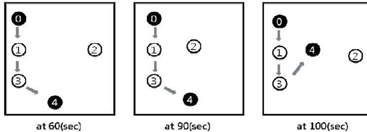
**Fig. 3. Routing Path of Original AODV during Moving Nodes.**
