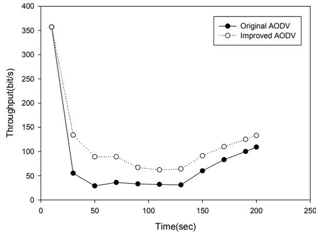
**Fig. 9. Comparison of Throughput when Moved Nodes Based on IEEE 802.15.4.**
