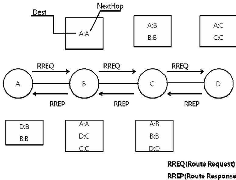
Fig. 1. AODV Routing Discovery.
