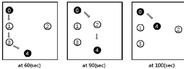
Fig. 4. Routing Path of Improved AODV during Moving Nodes.
