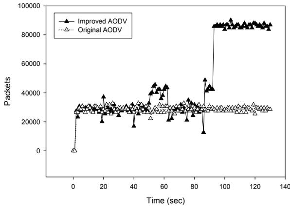
**Fig. 7. Comparison of Throughput when Moved nodes Based on IEEE 802.11.**
