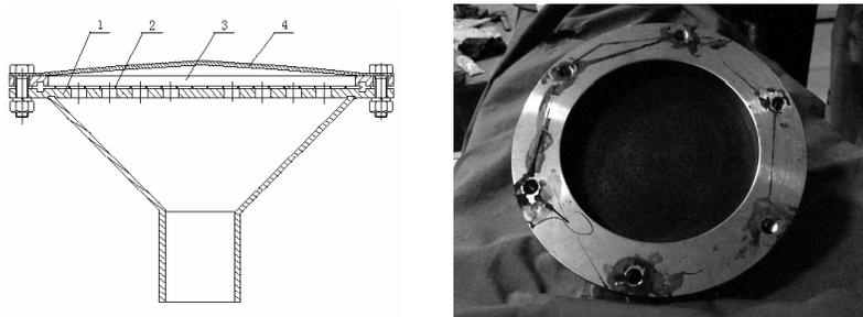
1. Sieve plate, 2. Membrane micropore, 3. Stainless steel plate, 4. Position-limit cover.
