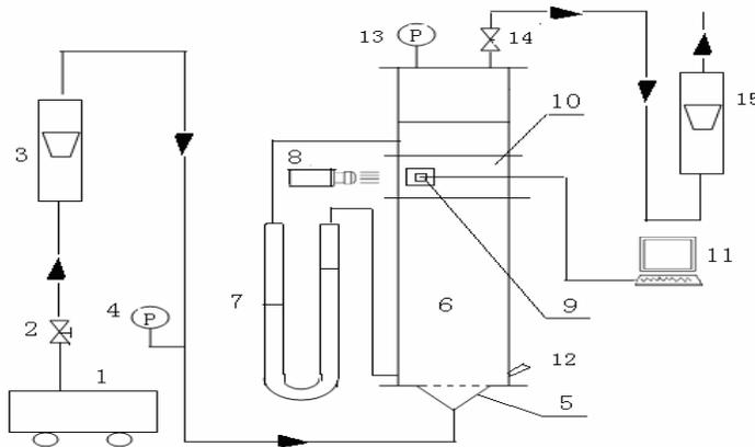
1. Compressor, 2. Pressure stabilization valve, 3. Inlet rotameter, 4. Inlet Manometer, 5. Membrane micropore aeration gas distributor, 6. Bioreactor, 7. U-shape differential manometer, 8. YAG laser system, 9. CCD camera, 10. PIV test section (water jacketed area), 11. Computer, 12. The portable oxygenic electrode, 13. Outlet manometer, 14. Outlet valve, 15. Outlet rotameter.
