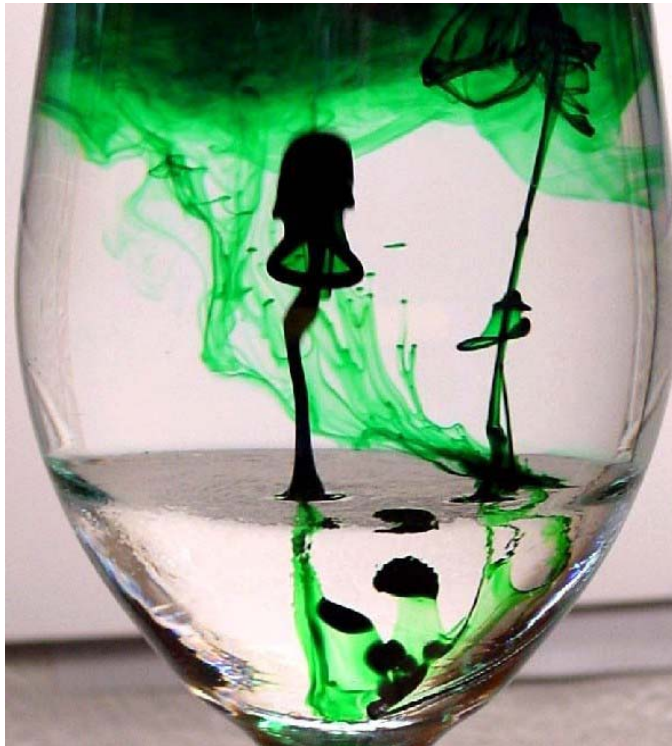
Fig. 1. Buoyancy through Interface. A Buoyant Jet of Dyed 70% Isopropyl Alcohol Rises through the Interface Formed by Corn Syrup and Water. [9]
