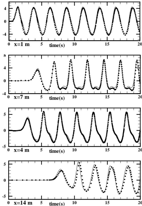
**Figure 3: Comparisons of the free-surface elevation for nonlinear sinusoidal wave propagation along the wave channel between numerical results (solid line) and experimental data (circles). The amplitudes are expressed in cm.**
