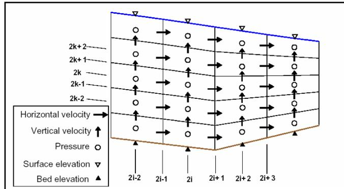
Fig. 1. Presentation of Staggered Grids and the Positions of the Variables.
