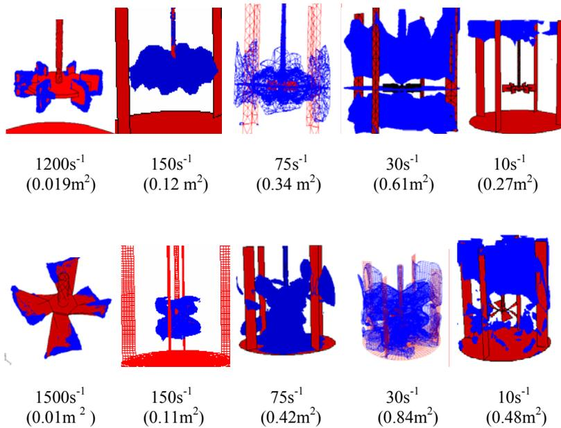
**Fig. 6. Iso-Zones Corresponding to Different Strain Levels At Viscosity 2Pa; Re=100. (The surface area indicated in brackets represents the relevant strain rate spatial distribution).**
