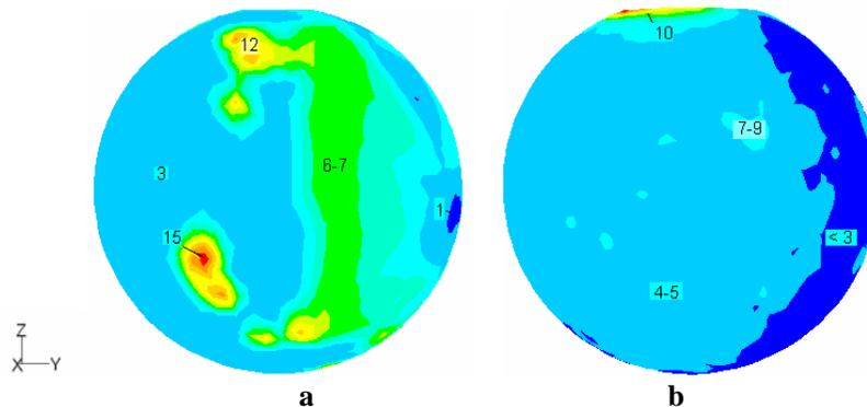
**Fig. 2. Simulation Set-Up and CFD Strain Rate Contours (in  $\text{ks}^{-1}$ ) Obtained at the Spherical Particle Wall by RT mixing at  $N=10$  rps in Cases of Water (a) and power law liquid ( $K=0.38 \text{ Pa}\cdot\text{s}^n$ ,  $n=0.26$ ) (b)  $\mu_a=12 \text{ mPa}\cdot\text{s}$ .**
