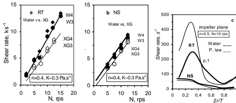
**Fig. 5. Selective Shear Rate (In  $\text{Ks}^{-1}$ ) Damping In Power Law Flow Affected By Impeller Design: Experimental Near-Particle  $\dot{\gamma}$  (a) (b) and CFD-Inner Flow  $\dot{\gamma}$  Profiles (c) Corresponding To RT And NS: A Qualitative Comparison.**
