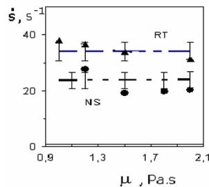
**Fig. 3. CFD Generated Relationships Of Volume-Averaged Shear Rates Vs. Dynamic Viscosity In Laminar Flow.**
