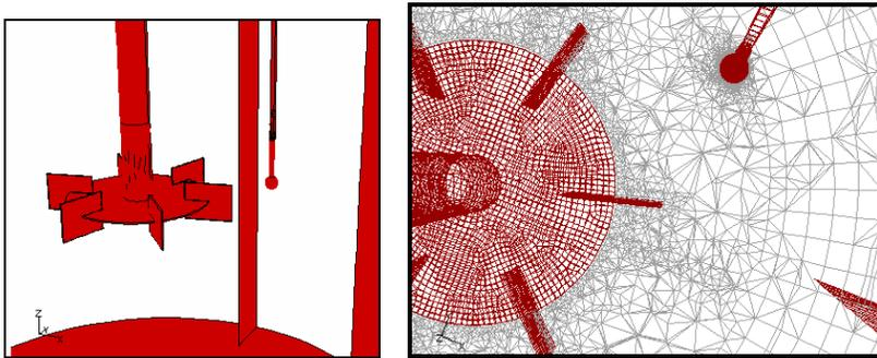
**Fig. 1. Experimental Set-Up for Measurement of Shear and Extended Mesh Refinement for its Simulation.**
