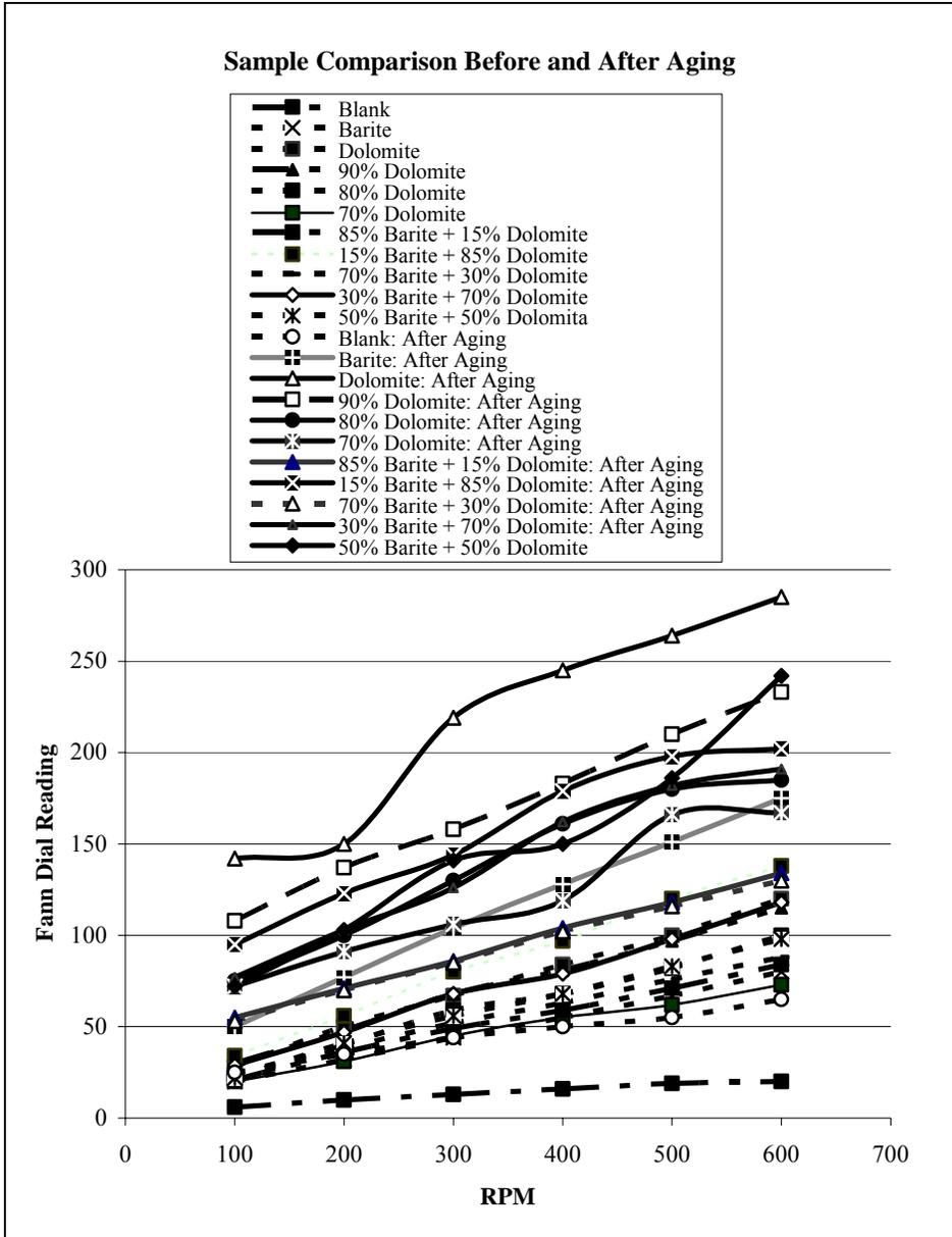
Fig. 6. Fan Samples Reading on the Viscometer Fan Cylinder before and after Aging.
