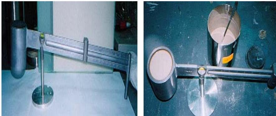
**Fig. 1. API Mud Balance Used in the Test.**
