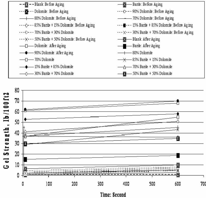
**Fig. 7. Gel Strength before and after Aging**
