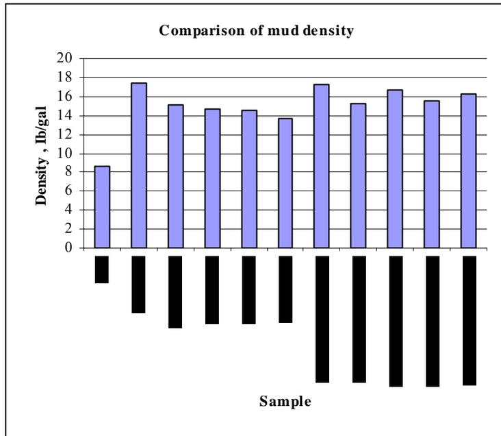
**Fig. 4. Mud Slurry Density at Various Compositions.**
