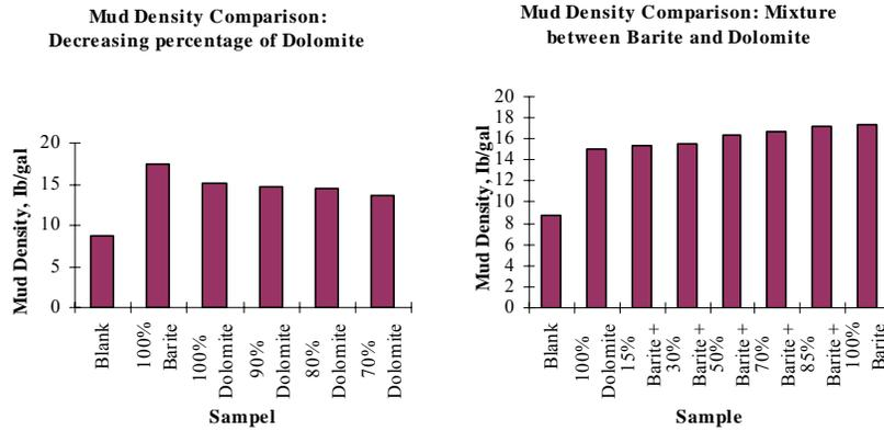
**Fig. 5. Slurry Density at Various Dolomite and Barite Content.**
