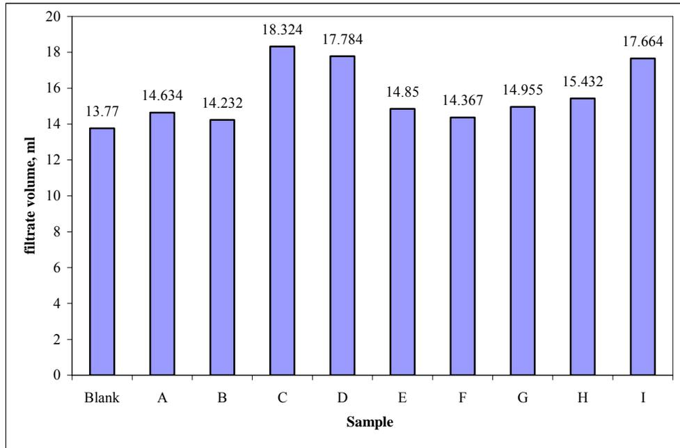
**Fig. 9. Filtrate Loss from HTHP Filter Press.**
