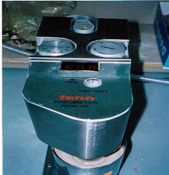
**Fig. 2. Fann Rotational Viscometer.**
