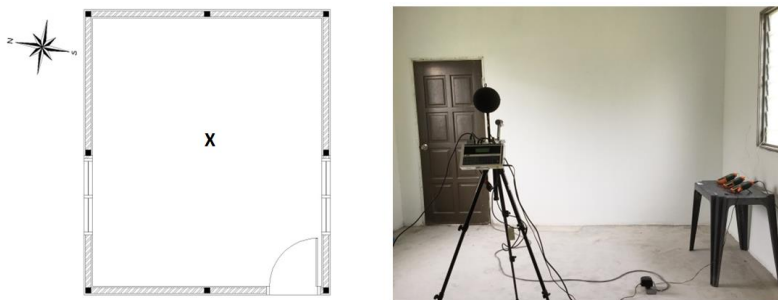
Fig. 5. Positions of sensors and data logger.
