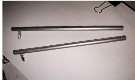
Fig. 3. Model of antenna dipole open \frac{1}{2} UHF broadcast. (b) Manufacturing results.
