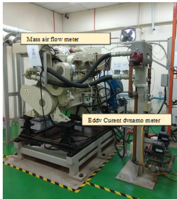
Fig. 1. Cummins NTA 855M 6-cylinder turbocharged marine diesel engine.
