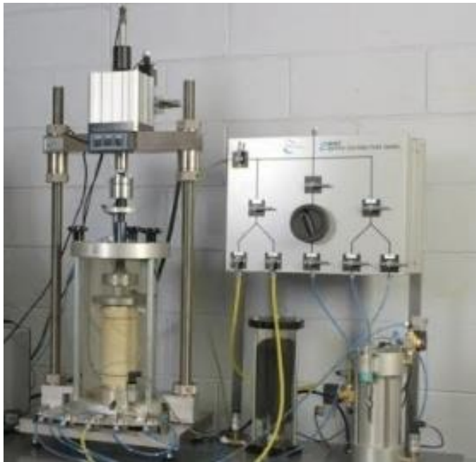
Fig. 3. Cyclic triaxial compression testing.
