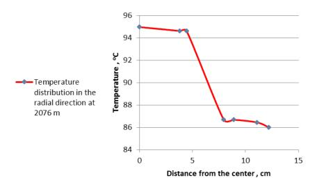
Fig. 8. The temperature distribution in the well wall and the surrounding at depth (2076 m)
