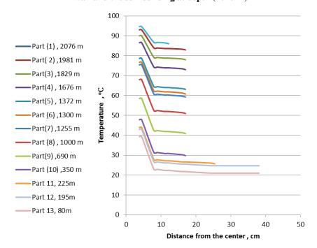
Fig. 9. The temperature distribution in the well wall and the surrounding at different depths.
