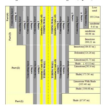
Fig. 5. Vertical section of the oil well and surrounding formation.
