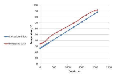
Fig. 10. Comparison between present calculated data and measured data (static case).
