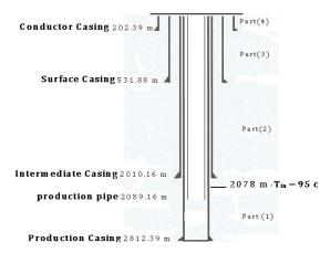
Fig. 4. Schematic well bore diagram (6Q1-59).
