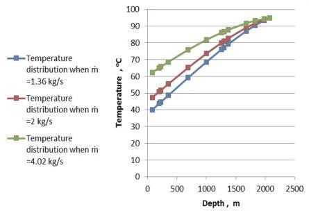
Fig. 11. Temperature distribution for different mass flow rates.
