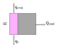
Fig. 3. Schematic of the heat-transfer in wellbore.
