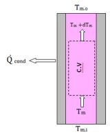
Fig. 2. control volume for internal flow in oil well.
