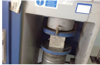
Fig. 1. Compressive strength testing machine.
