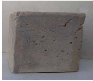
Fig. 3. Studied concrete cube (200×200×200) mm 3 .
