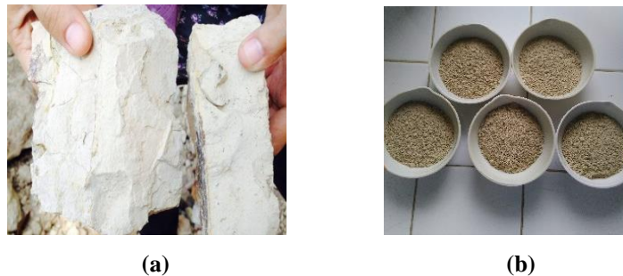
Fig. 1. Samples of the adsorbent: (a) Natural bentonite before the activation process; and (b) Bentonite after the activation process.
