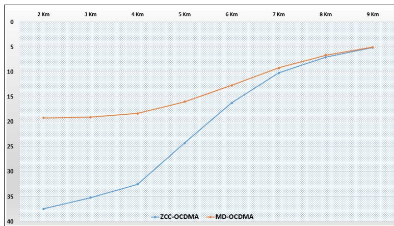
Fig. 9. Q-Factor results of 1D zero cross correlation and 1D multi diagonal codes over different MMF distances.
