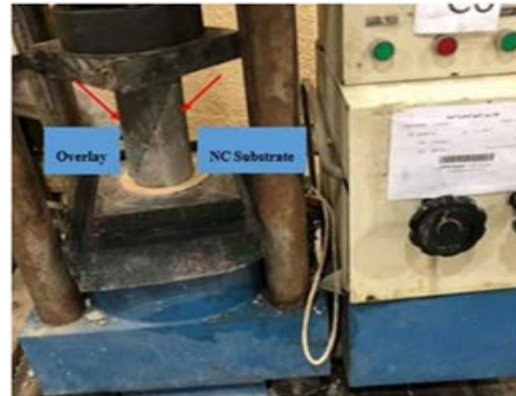
Fig. 4. Test setup for slant shear test.
