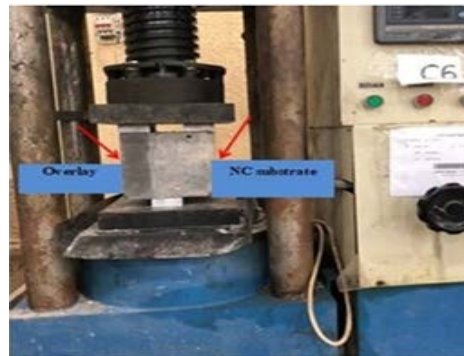
Fig. 5. Test setup for bi-surface shear test.
