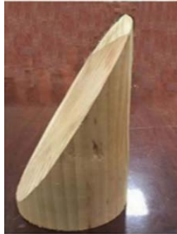
Fig. 2. Wood slices for slant shear test.
