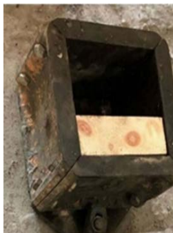
Fig. 3. Wood slices for bi-surface shear test.
