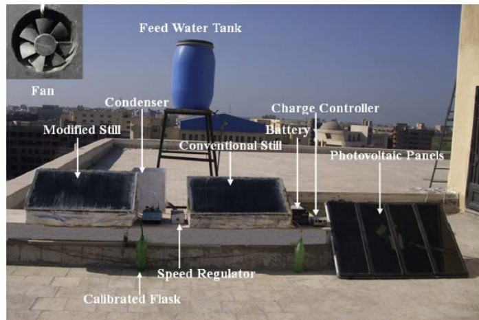
Fig. 15. Photograph of the two conventional and modified solar stills (Kabeel et al. [88, 89]).
