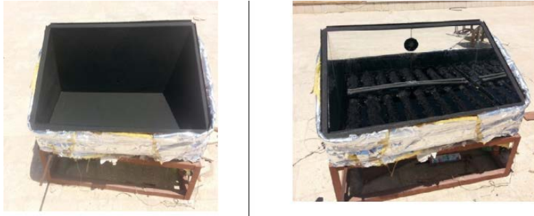
Fig. 20. Photograph of the two conventional and corrugated wick solar stills (Omara et al. [95]).
