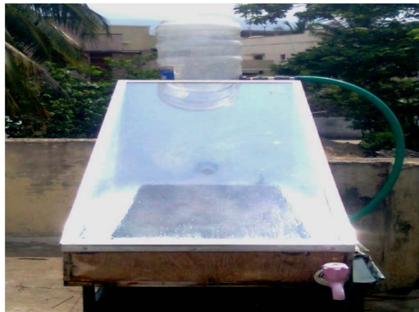
Fig. 5. The modified vacuum single basin solar still (Gnanadason et al. [76]).
