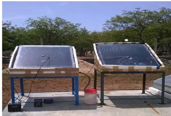
Fig. 8. Photograph of the single basin single slope solar still (Elango et al. [79]).
