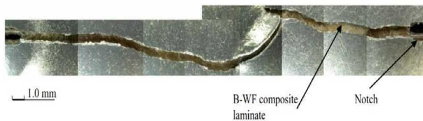
Fig. 10. The crack growth on the aluminium laminate of the FMLs.
