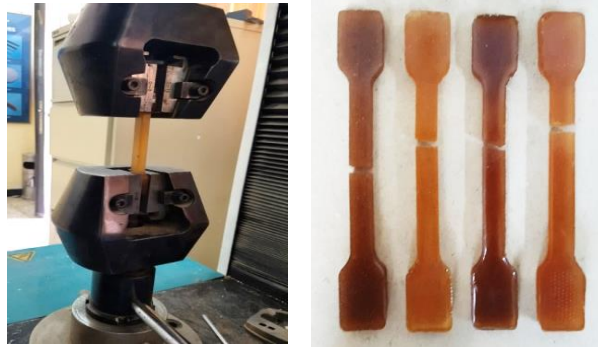
Fig. 8. Tensile device and the failed samples after tensile test of PS/epoxy composite.
