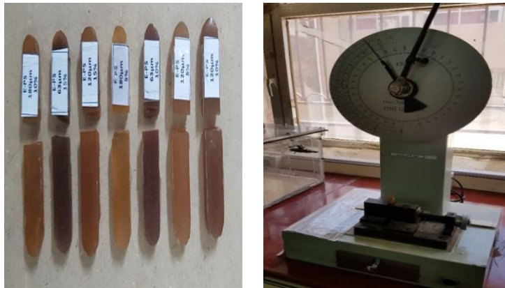
Fig. 14. Impact device and the failed samples of the impact test.
