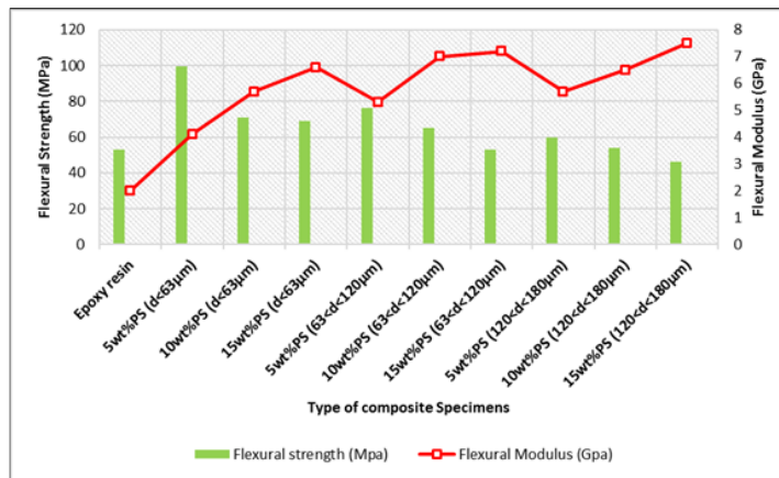
Fig. 12. Type of composite specimens versus flexural strength and flexural modulus.
