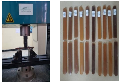
Fig. 11. Flexural device and the failed samples.
