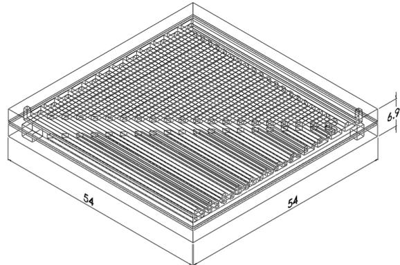
Fig. 2. Dimensions of fuel cell stack in mm.
