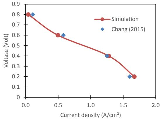
Fig. 3. Validate simulation results with experiments.
