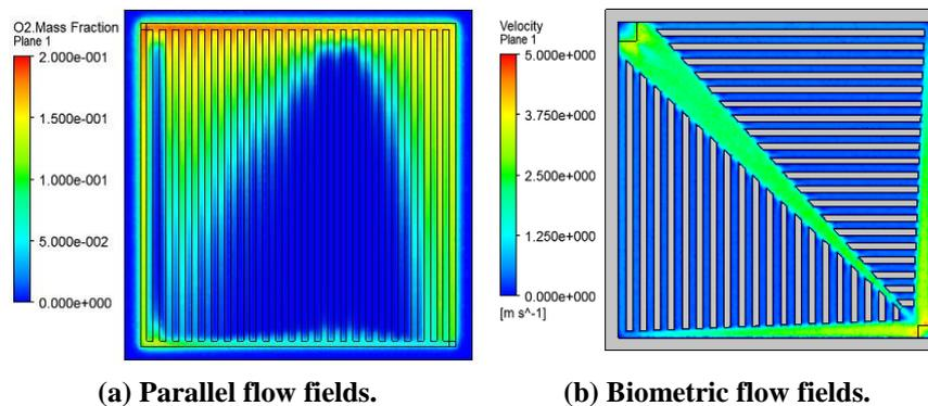
**Fig. 5. Distribution of oxygen concentration in cathode diffusion layer.**
