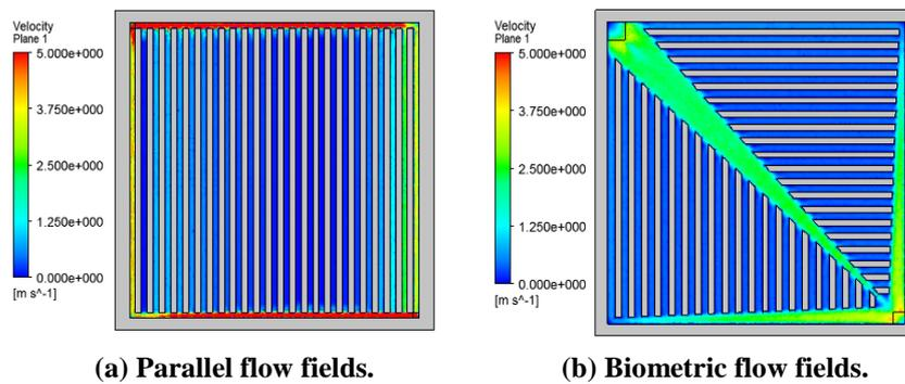
Fig. 4. Distribution of oxygen velocity in cathode side.
