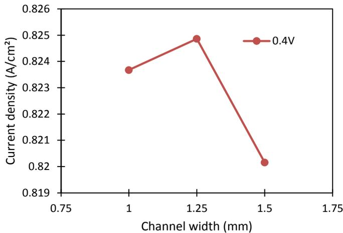
Fig. 7. Graph of current density at 0.4 V with variations in channel width on biometric flow field.
