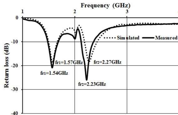
(a)  $|S_{11}|$  characteristics for proposed Antenna-II when  $L_i = 35$  mm.
