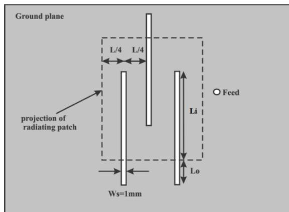
**Fig. 2. Top view (ground plane).**
