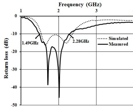
**Fig. 6.  $|S_{11}|$  characteristics for proposed Antenna I when  $L_i = 35$  mm.**
