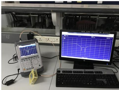
**(b) Testing on vector network analyser.**
