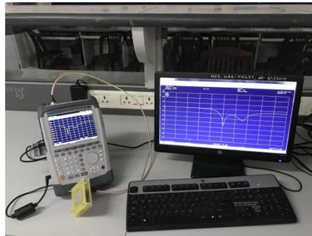
(b) Testing on vector network analyser.
