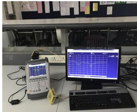
(b) Testing on vector network analyser.
