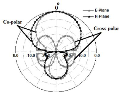
(c) E-plane and H-plane radiation pattern at 2.5 GHz.
