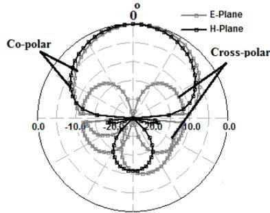
(b) E-plane and H-plane radiation pattern at 2 GHz.
